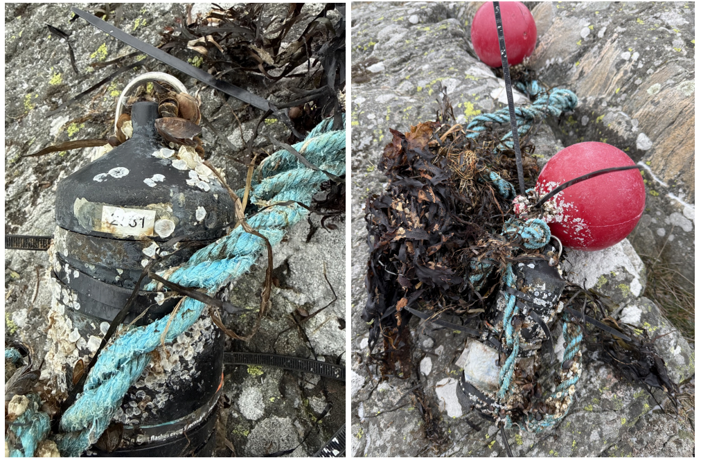
Figure 2: Acoustic receiver initially deployed in Danish waters, found on a Swedish beach.
